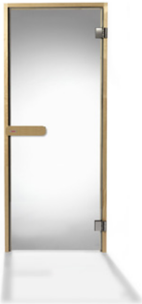
All-glass door for the commercial sauna area With an opening width of 74 cm; suitable for wheelchairs. 8 mm safety glass, alternatively clear or bronze-tinted.
